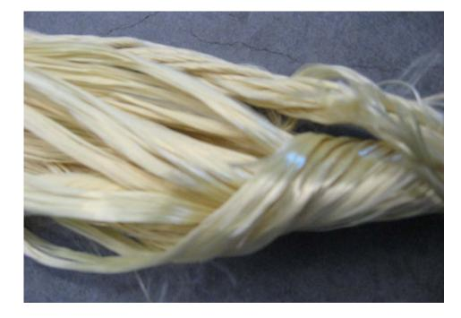
Super Aramide before test, breaking strength 20.000 kg
